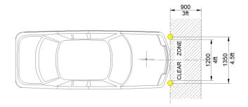
Note at 6.5ft/2000mm bollard spacing at 25° impact angle, the clear zone extends 3.5ft/1077mm perpendicular to the string of bollards. While the potential for vehicles to breach the string of bollards would follow a saw tooth pattern, the 3.5ft/1077mm clear zone offset should be applied to the entire length of the bollard string.
