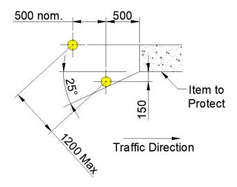
Note the 3ft/900mm clear space between the centre of the bollards and the "protected item". The potential angle of impact is set at 25 degrees, this can be adjusted as required by the designer, considering the likely angle of impact at the site.
