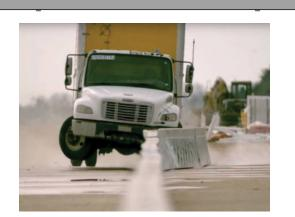
With patented hybrid technology and unique connectors, the HV2 Barrier offers high containment and low deflection upon impact, while remaining economical to transport and deploy.
