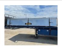
On full loads, secure the 3 tie downs per row, evenly spaced. As a guide, place each chain in the position as illustrated on the picture below (evenly spaced).
