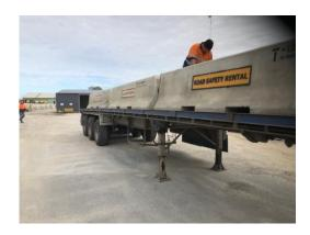
10.14 To secure the load, use 2 chains per row of T-Lok with chains rated to 30T.
