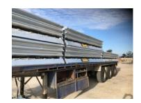
Begin loading the second stack of barriers as per the same loading method as the botton stack Ensure when you are stacking the barriers they lock into the bottom layer. Saferoads barriers have been purposely designed so they will stack neatly which will resist any movement in transit.
