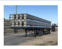
On full loads, secure the 4 tie downs per row, evenly spaced. As a guide, place each strap in the position of the concrete blocks in the barrier
