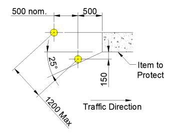
Note the 20in/500mm clear space between the centre of the bollards and the "protected item". The potential angle of impact is set at 25 degrees, this can be adjusted as required by the designer, considering the likely angle of impact at the site.
