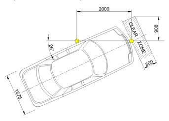
The spacing of the bollards can be altered depending on the design impact angle and allowable clear zone behind the string of bollards.
