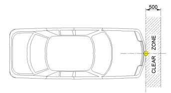
When designing bollard arrays, or strings, the direction of all potential impacting vehicles needs to be considered to ensure the design is fit for purpose.
