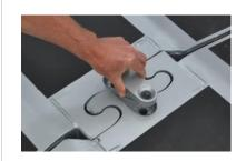
Place the machined joining plate into the designated position.
