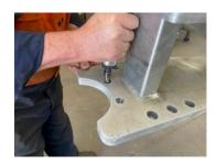
Once this has been tightened using the air impact wrench, ensure that the bearing spins freely.
