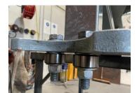
Repeat the process with the second M20 bolt / washer and bearing assembly and tighten.
