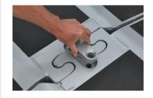
Place the machined joining plate into the designated position.
