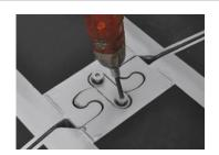
Using 2 x M20 countersunk bolts and a 12mm hex key, install the joining plate into the bollard connectors.
