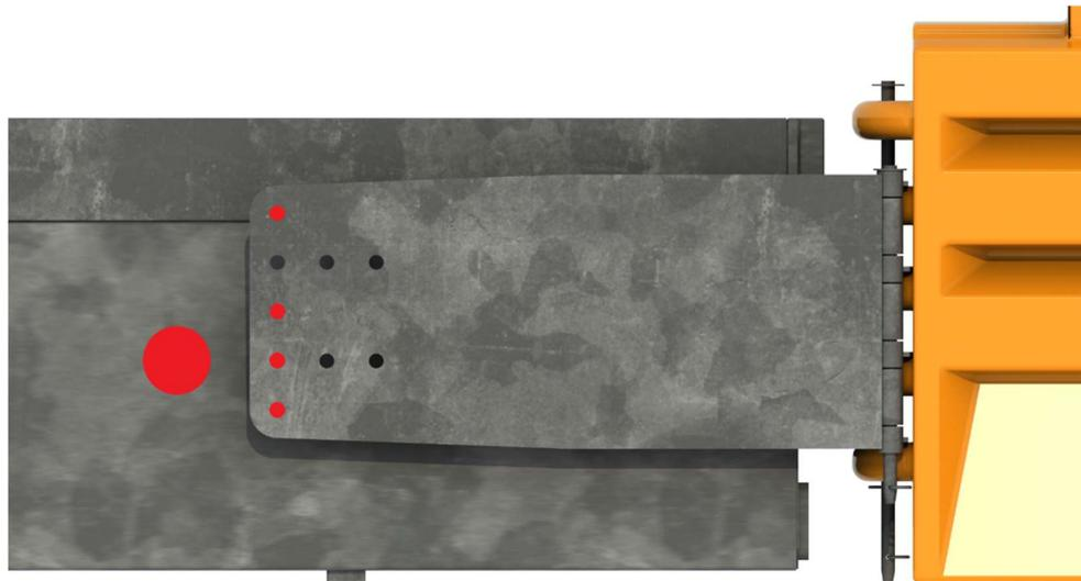
3. Attach the transition panels to the HV2 Barrier using eight M20 x 75mm hex head bolts and nuts. The hex heads are to be on the outside face of the transition plates.
