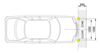
Note at 6.5ft/2000mm bollard spacing at 25° impact angle, the clear zone extends 36in/908mm perpendicular to the string of bollards. While the potential for vehicles to breach the string of bollards would follow a saw tooth pattern, the 36in/908mm clear zone offset should be applied to the entire length of the bollard string.
